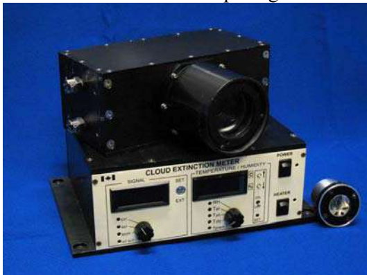
Figure 2. Cloud Extinction Probe: optical unit (top); control box (bottom); retroreflector (right).
