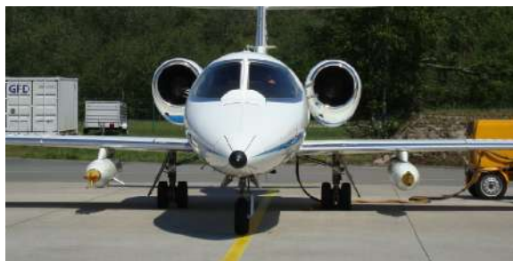
Fig.7. UFT-2 in housing attached to the container under the left wing of Learjet aircraft.
