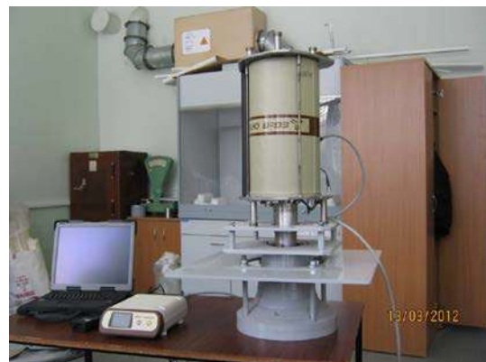
Fig. 14. Gamma spectrometer with scintillation and high purity germanium detector GEM 40-86 «ORTEC»
