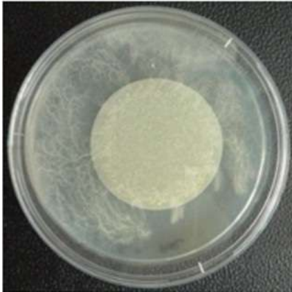
Fig. 2: Agar plate with AIDA filter sample of soil dust particles after cultivation at 20°C (courtesy of A. Rieder)
