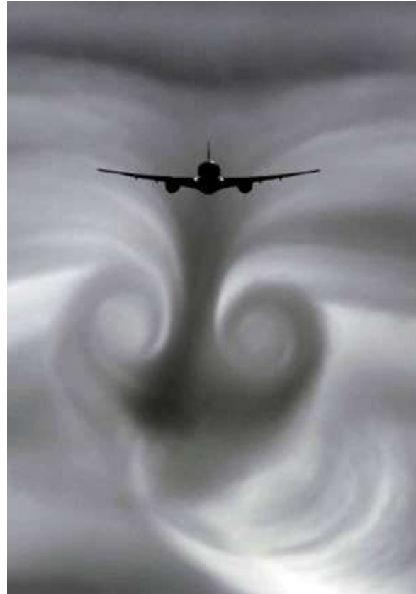
Fig. 2. Downwash and vortex pair below a B-777-200 aircraft (mass \sim 145000 kg) flying immediately above a 150 m thick cloud while approaching London Gatwick airport at 7AM local time on 10 July 2006. Surface temperature was 16^{\circ}\text{C} . Aircraft was descending through 0.61 km altitude at a speed of \sim 108 m/s. Photograph courtesy of Steve Morris photographer, who was positioned \sim 9 km in front of the approaching aircraft at the surface, using a 840mm telephoto lens. Cloud in this viewing area was reported to completely dissipate 20 minutes after the photograph was taken.
