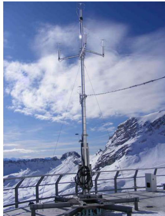
Figure 6. The mast of ultrasonic wind sensors on the roof of UFS.
