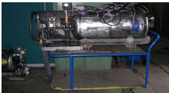
Fig. 21. The small ice particle generator SIPG-A
