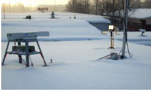
Figure 1. PVI installation at the University of Helsinki precipitation measurement site in Järvenpää.
