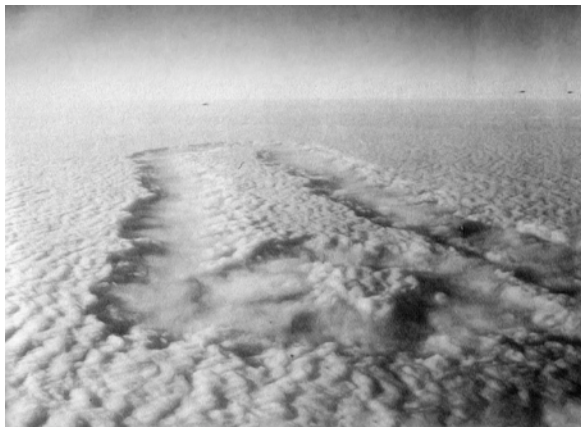
Fig. 1. "Racetrack" cloud dissipation pattern photographed 24 minutes after a B17 aircraft completed flying the pattern immediately above cloud top at 2070m ASL for 13 minutes at a speed of 76 m/s. The temperature at the top of this 700-m thick cloud was -5.6^{\circ}\text{C} . The longer sides of the oval shape are about 29 km long, and the path cleared is 2-3 km wide. Crushed dry ice pellets with diameter 5-10 mm were dispensed through a small hole in the B17 floor at a rate of 480 g/km. Picture was taken at 11:21AM local time on 24 Nov 1948 over Utica NY. Note that dissipated cloud did not penetrate to cloud base, even though the entire depth of the cloud was < 0^{\circ}\text{C} .
