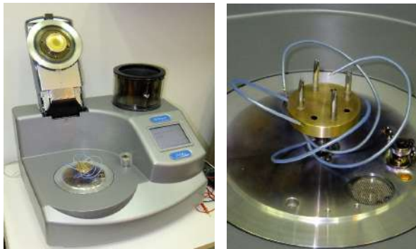
Fig.2. Four UFT-2 sensors ready for coating with gold in a special clamp in sputter coater.
