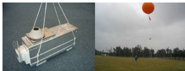
Figure 1. Videosonde (left) and launching balloon (right). Videosonde used in this study was an improved version of that designed by Takahashi (1990). 450(L)x150(W)x220(H), 1.7kg.
