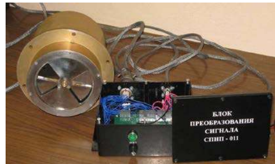
Fig. 23. Aircraft electrical field mill SPNP-011
